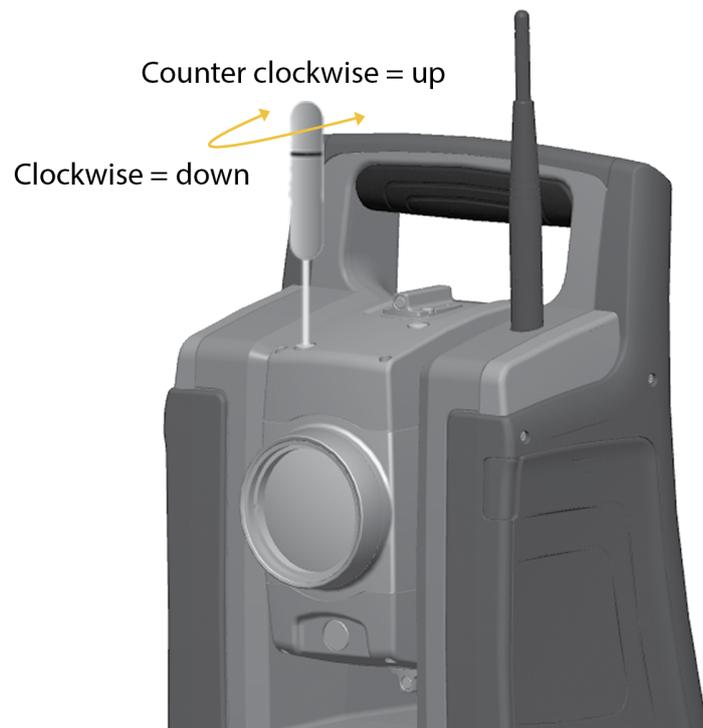
To correct the horizontal position of the laser spot, insert the allen key into the horizontal adjustment port and turn it as shown:
