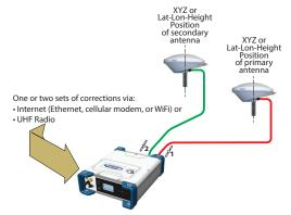
On the receiver's General Status screen, the receiver will display "FIXED" (with short "FLOAT" transition time) when computing a position in RTK mode for the primary antenna.
