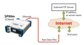
The receiver being the client for this transfer, you need to enter the IP address (or host name) and IP port of the remote FTP server, and also enter the login and password that will let the receiver upload its files to the server (see **Receiver**> **Sessions> External FTP Servers** on the Web Server).
