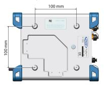
Preparing the support on which the receiver will be mounted only consists of drilling four holes, forming a simple, 100-mm square. In the receiver case, the four tapped holes are designed as follows:  $M4 \times 0.7 - 7$  mm. When tightening M4 screws, the recommended torque is 2.6 N.m (23 lfb.in).
