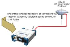
On the receiver's General Status screen, the receiver will display "FIXED" (with short "FLOAT" transition time) when computing a position in Hot Standby RTK mode. The computed position is displayed after pressing (?...).
