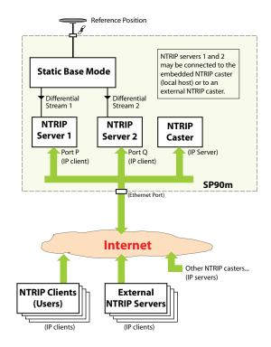
In its simplest configuration, the embedded NTRIP caster can be used to emulate the Direct IP mode (i.e. IP connection to a unique source of corrections), with the additional advantage that, contrary to conventional Direct IP, the embedded NTRIP caster can offer an effective protection of the source of corrections by restricting its access to the sole authorized users.
