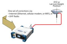
On the receiver's General Status screen, the receiver will display "FIXED" (with short "FLOAT" transition time) or "DGPS" when computing a position respectively in RTK or DGPS mode.
