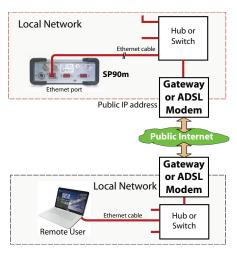
In this configuration, the IT expert should take all the necessary steps for the receiver owner to be able to access the SP90m through the public IP address of the local network. In this case, the IP address shown on the receiver display screen is NOT the one to be entered in the web browser.
