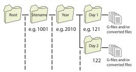
Organizing the storage of the files is simply obtained by typing the appropriate codification of the subdirectories in the field named **Sub-directory Name Format**. This field uses a specific syntax with case-sensitive characters. A typical syntax used is the following:
