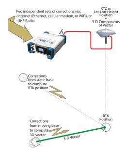
On the receiver's General Status screen, the receiver will display "FIXED" (with short "FLOAT" transition time) when computing a position in RTK mode. The computed RTK position is displayed after pressing . A new press on this button will display the computed components of the vector.
