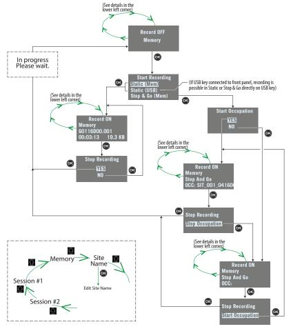
The Record screen being displayed, press the down-arrow key to access the following parameters:
