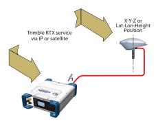
Using a Trimble RTX service in the SP90m requires that you first buy a subscription to this service. On the other hand, the receiver is ready to operate in Trimble RTX mode (dedicated firmware option has been pre-installed at the factory) provided an L-band capable GNSS antenna is used.
