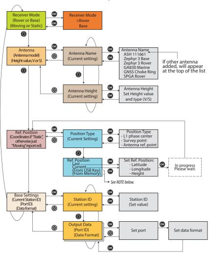
NOTE: For a static base, the reference position can also be imported from a USB key connected to the receiver's USB port via the short OTG cable. The USB key should contain one or more properly formatted csv files, each containing one or more site positions. For more details see page 43.
