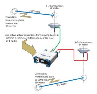
To configure the receiver as a Dual Relative RTK rover, use the Web Server as follows:
