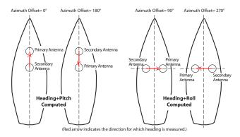
For each of these setups, if you enter the indicated azimuth offset, then the receiver will deliver the vehicle's true heading, and not the heading value it actually computes.
