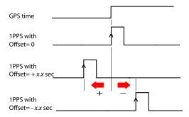
Active edge, i.e. the edge (falling or rising) synchronized with GPS time. (On the diagram above, it is the rising edge that is set to be the active edge).
