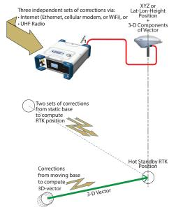
On the receiver's General Status screen, the receiver will display "FIXED" (with short "FLOAT" transition time) when computing a position in Hot Standby RTK mode. The computed position is displayed after pressing .
